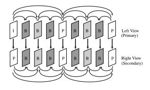
Fig. 1. Typical MVC structure for stereoscopic video.
